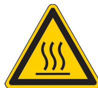
Caution: Hot surface
